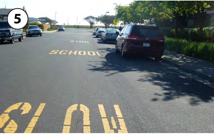
SLOW SCHOOL XING pavement stencils signal that an uncontrolled crosswalk is ahead.
