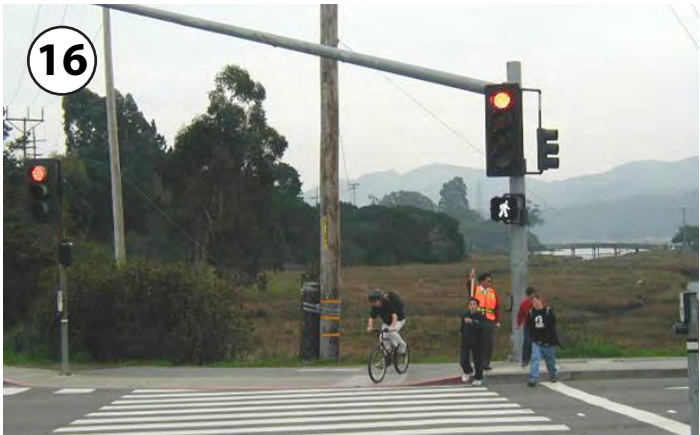
Leading pedestrian interval phasing allows pedestrians a head start crossing the street.
