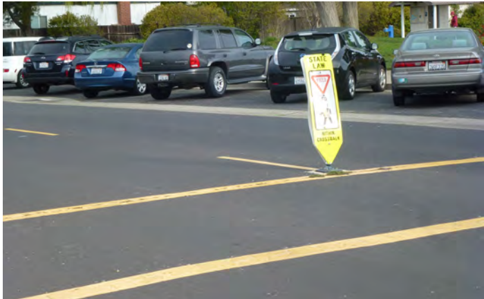
In-street signage at the uncontrolled crossing on Niantic Drive increases visibility.
