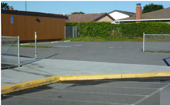
Passenger loading zones should be demarcated with white curb paint.
